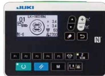
The sewing machine can be paired with equipment which supports NFC (Near Field Communication) only by holding the equipment over the sewing machine.
