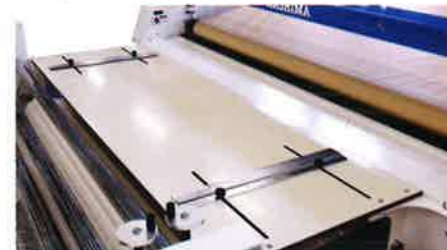
The Table and Paper guide assists to install the materials in to the machine
