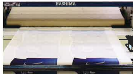
Installation of the material from above makes the printed surface on the transfer paper to adjust with the materials.
