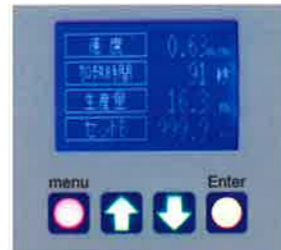
LCD Panel shows, Speed, Heating time, and production quantity.
