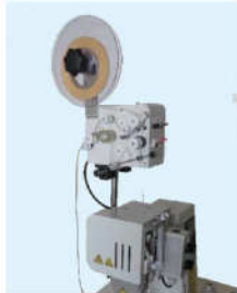
OP : Tape releaser for release paper
